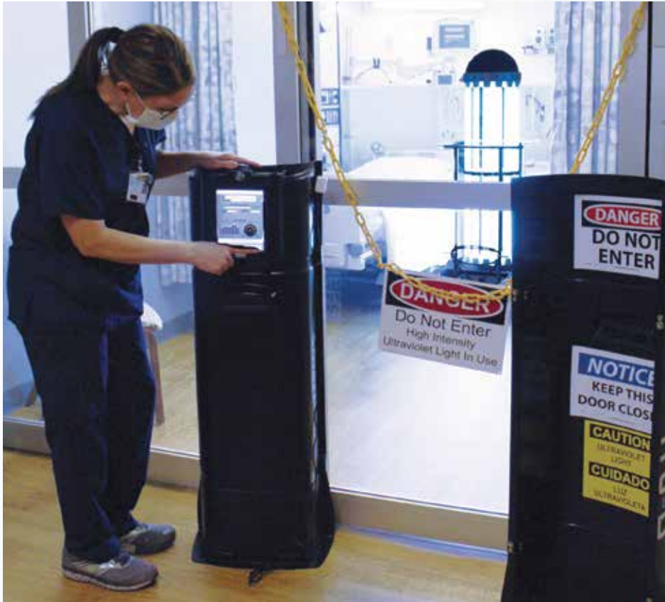
Dawn DeHollander, an FCHC Environmental Services Technician, adjusts the Tru-D ultraviolet sterilizing unit, which provides added infection prevention.
