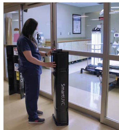
Heather Mitchell, Environmental Services Tech II, operates a high-tech Tru-D® SmartUVC unit that uses high intensity ultraviolet light to inactivate bacteria and viruses in the Emergency Department.
